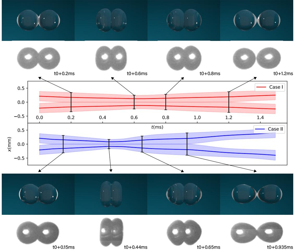
Figure 10: Time evolution of the binary droplet collision for Case I and II. Top and Bottom: Representative frames of the rendered images from our simulation and the experimental snapshots from Pan et al. [2008]. Middle: The evolution of the  $x$ -axis positions of two droplets. The regions filled by the light color are the  $x$ -axis bounding box of two droplets. Solid lines denote the  $x$ -axis center position of two droplets.
