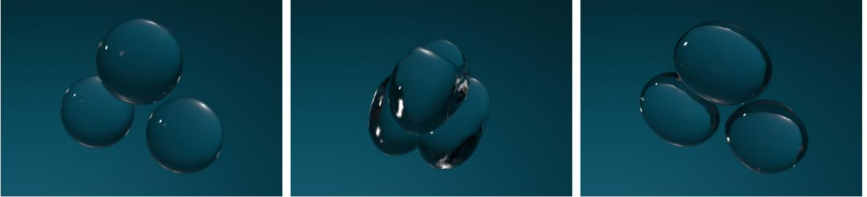
Figure 11: Time evolution of the trinary droplet collision, where three droplets collide, form a non-manifold gap between them and subsequently rebound.
