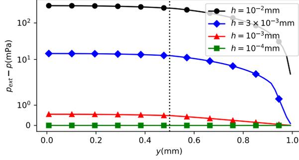
Figure 8: The pressure transmission in Figure 7 (Middle) with different air film thickness  $h$ . The pressure loss along the vertical lines at  $x = 0.5$  mm is plotted.
