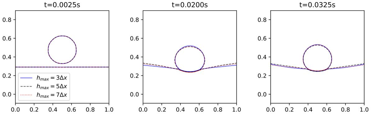
Figure 9: A 2D droplet falls on the liquid bath with different air film height thresholds  $h_{max} = 3\Delta x, 5\Delta x, 7\Delta x$
