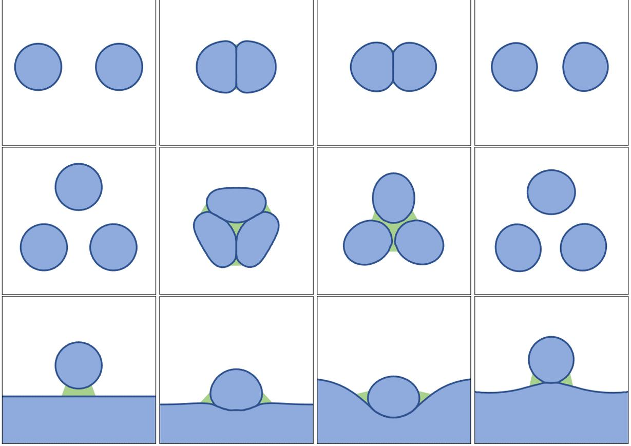
Figure 5: Time evolution of the 2D binary droplet collision (Top row), the 2D ternary droplet collision (Middle row), and the 2D bouncing droplet (Bottom row). Liquid volumes (blue) are visualized and air films (green) are depicted in the latter two examples.
