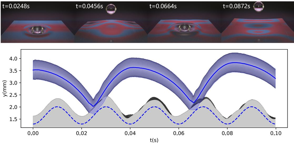
Figure 12: Time evolution of a droplet bouncing on a vibrating bath in  $(2, 1)$  mode. Top: Rendered images of four representative frames. Bottom: Temporal evolution of the scene. The solid line denotes the movement of the droplet center, and the dashed line denotes the bath movement. The background image is generated by stitching the successive simulation frames, where a cropped vertical section represents each frame through the droplet center.
