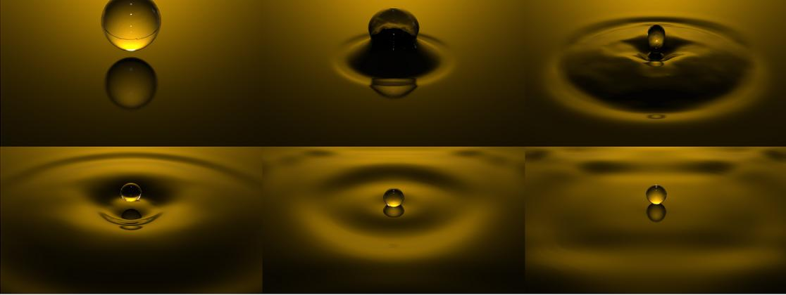
Figure 15: Droplet merging and pinching. A large droplet falls and merges with the bath, which causes a thin liquid column to form due to the surface tension. The column eventually breaks off and pinches off a smaller droplet bouncing on the bath.
