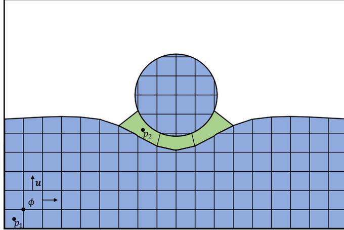
Figure 2: *Discretization of liquids and the air film.* The liquid domain  $\Omega_1$  (blue) is divided into several separate liquid volumes on the Cartesian grid enhanced by cut-cells, with level set  $\phi$ , pressure  $p_1$  and velocity  $\mathbf{u}$  sampled on nodes, cells, and faces. In the gap between liquid volumes, the air film  $\Omega_2$  (green) is represented by single-layered irregular cells and the cut-cell meshes to solve pressure  $p_2$ .
